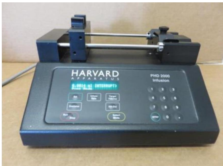
Fig. 55. Harvard Apparatus PHD 2000 syringe pump.
