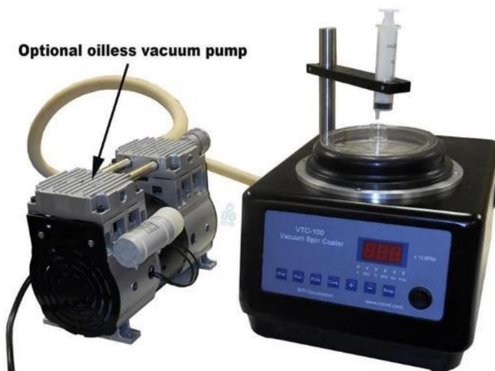
Fig. 53. Spin coater MTI Corp. Model VTC-100.
